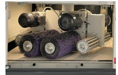
Equipped with 4 abrasive brushes and 4 spring wire brushes for edge rounding and oxide removal
