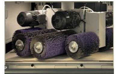
Equipped with 8 abrasive brushes for edge rounding
