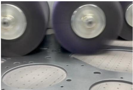
Edge rounding up to radius 2mm
