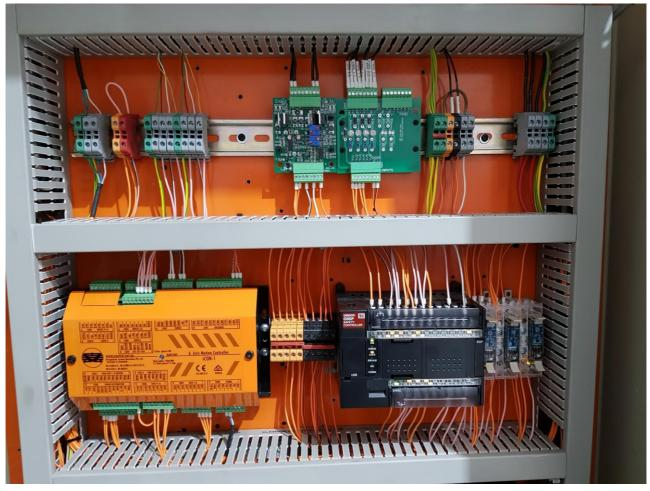
Omron Safety PLC - Programmed by CP Machinery
