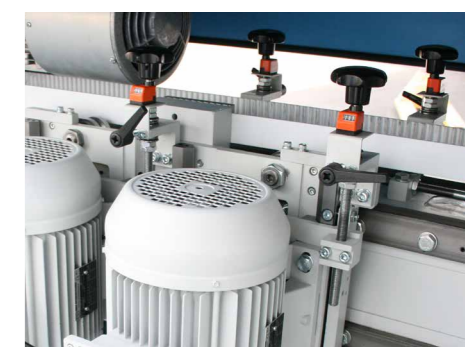
Separate height adjustment of each individual disc for quick compensation of tool wear
