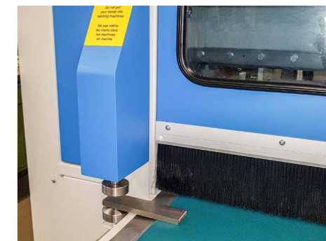
Motorized height adjustment, automatic setting of thickness using a limit switch (optional)
