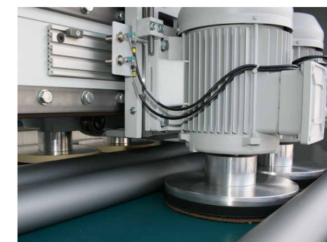
Four rotating discs with full-width oscillation for uniform 360° processing
